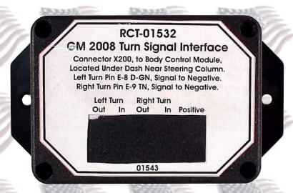
Left and Right Output Rated 12 VDC at 20 Ampere
