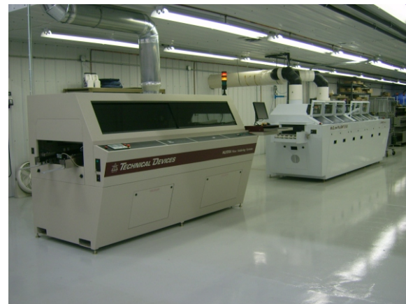
Computer Controlled Wave Solder Machine, Automatic Board Washer
